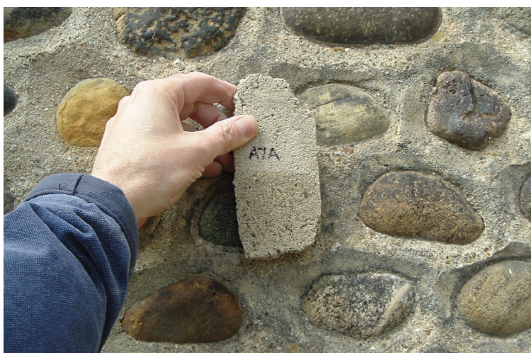
Fig. 6 (above) Examining a mortar sample.
